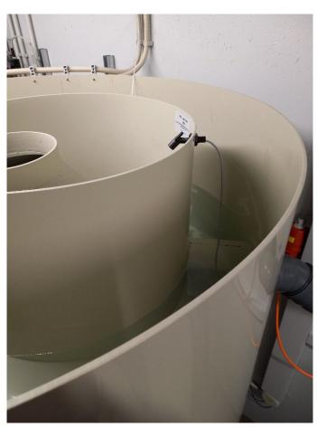
The ClearFox® DAF is a fully automated unit. The wastewater to be treated is fed from the customer's surge tanks or the ClearFox® buffer tanks of the DAF via a non-clogging cavity pump. The use of aerated buffers is recommended for certain applications.
